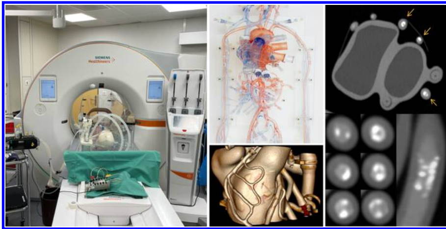
Figure 1. Overview of the cardiovascular phantom. The phantom setup on the CT scanner table is shown on the left. A close-up picture of the heart is shown in the middle together with a volume rendered CT image in the lower left part. A representative CT image of the heart is shown on the top right, whereby calcified plaques in the coronary artery wall are marked with small orange arrows. Close-up short- and long-axis images of a coronary plaque are shown in the lower right part of the figure.
